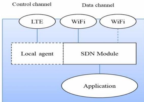
**Fig.1.4 SDN Wireless node internals**
