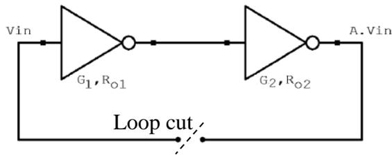
Fig. 4 Illustration of loop gain for a latch.
