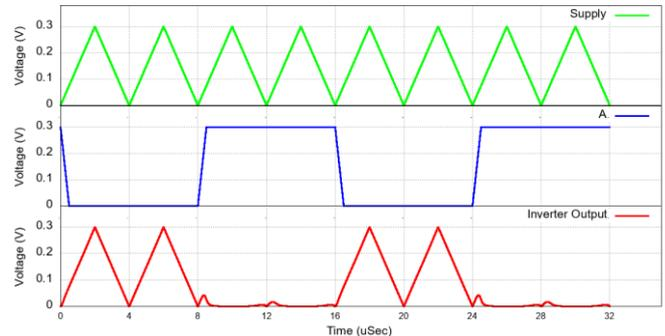
**Fig.14 Input output waveform for an inverter of SC-PFAL family.**
