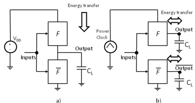
**Fig. 1 The energy flow in a) conventional CMOS logic and b) Adiabatic logic.**
