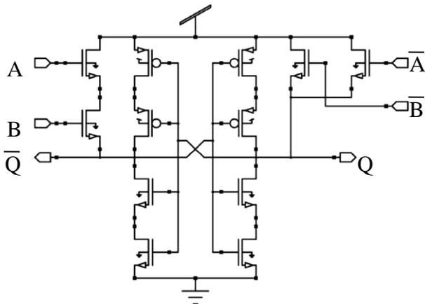
Fig.10 SC-PFAL two input NAND gate.
