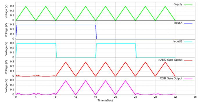
**Fig.15 Input output waveform for a two input NAND gate and a two input XOR gate of SC-PFAL family.**
