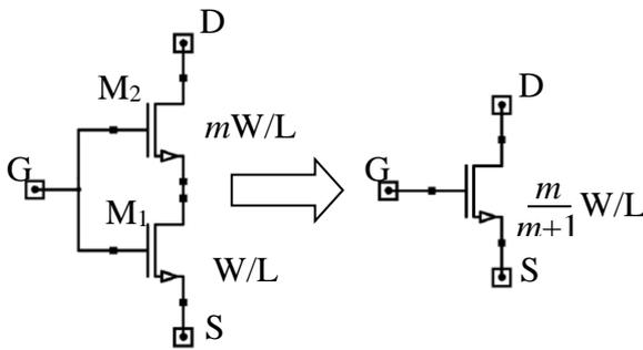
Fig. 2 Self Cascode Transistor.
