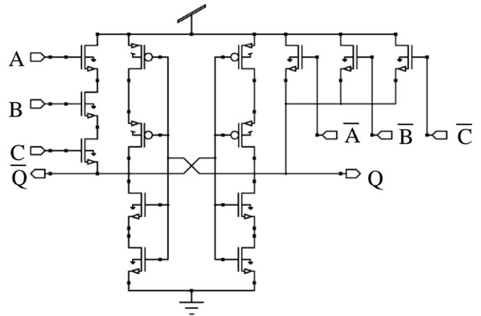
Fig.12 SC-PFAL three input NAND gate.
