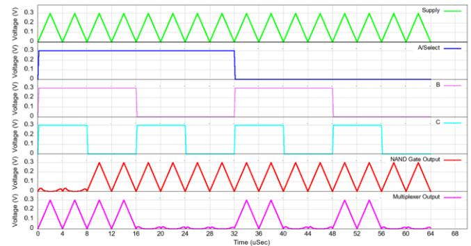
**Fig.16 Input output waveform for a three input NAND gate and a Multiplexer of SC-PFAL family.**
